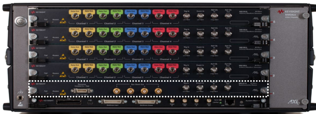
Figure 8. M8197A, front panel view and system with 16 synchronized channels (4x M8195A modules and 1x M8197A module).
