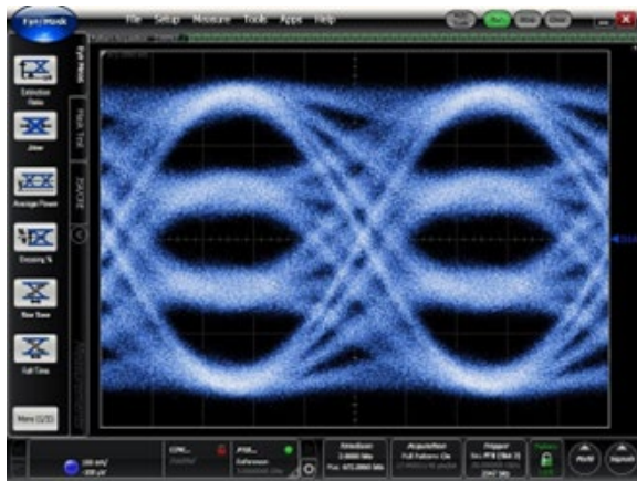
Figure 2. 4 PAM4 signal at 28 GBaud (= 56 Gbit/s).
