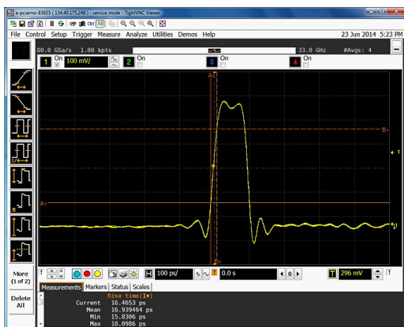
Figure 6. 100 ps pulse with 17 ps risetime.
