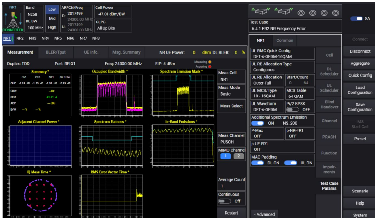
Figure 13. 5G NR FR2 RF measurement results example
