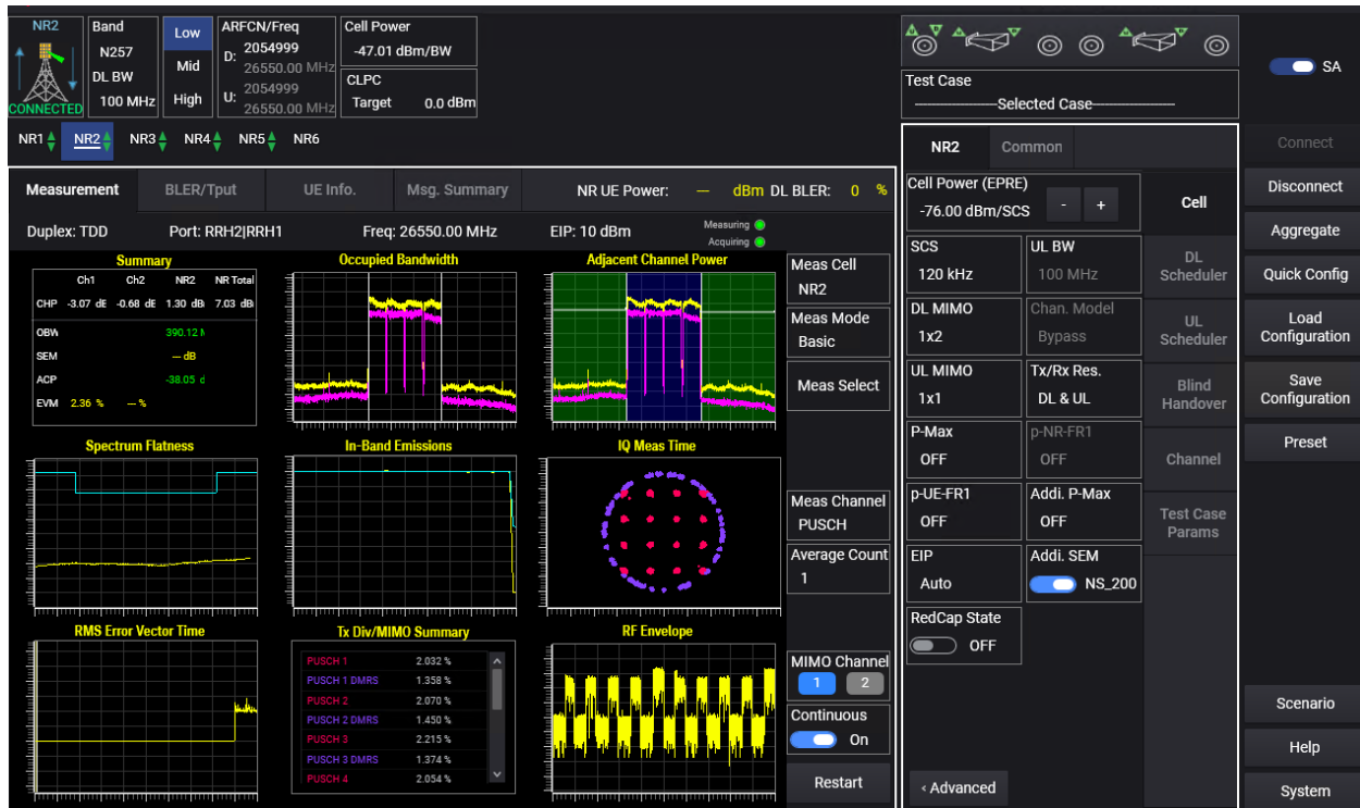
Figure 11. NR-DC connection and measurement
