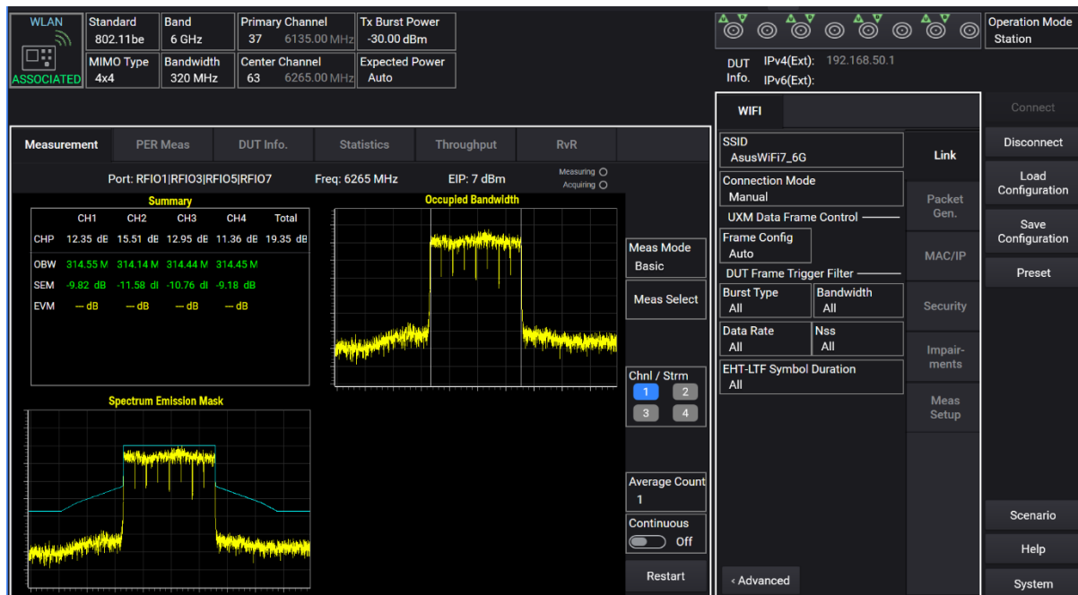
Figure 20. 802.11be 320 MHz bandwidth with 4x4 MIMO testing example
