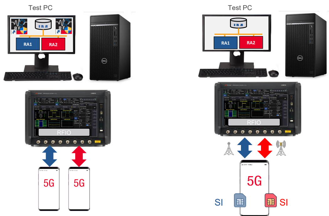
Figure 5. Dual UE (left) and Dual SIM (right) testing with S8702A RF Automation toolset.
