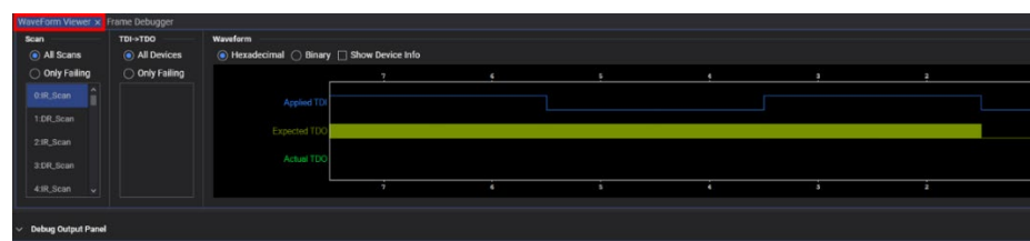
Figure 16. Waveform viewer shows the expected and actual values of the TDO signal for the test.
