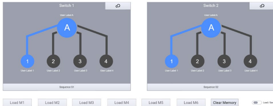
Figure 7. Web GUI of N7731C: two 1 x 4 switches
