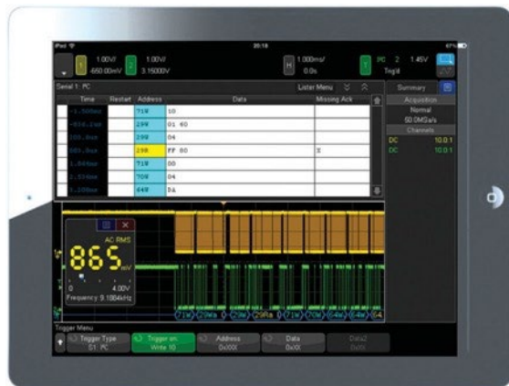
Figure 37. Tablet virtual front panel control.
