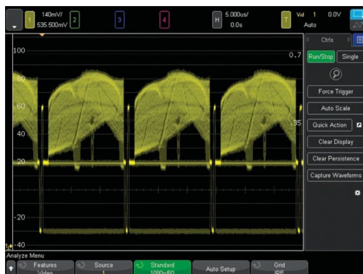
Figure 27. Triggering on 1080p HDTV signal analysis.
