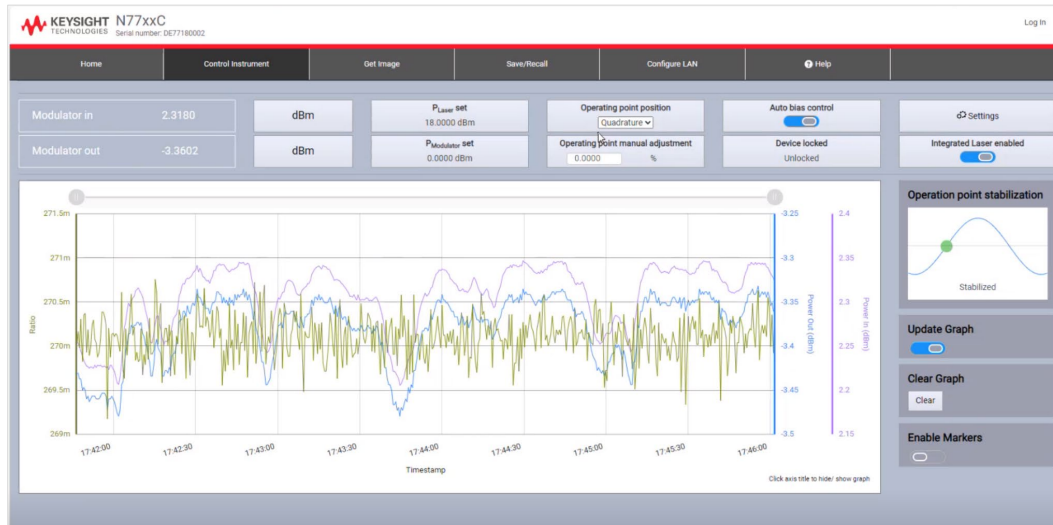
Figure 4. Bias control in N7718C user interface: output/input power ratio at quadrature point.
