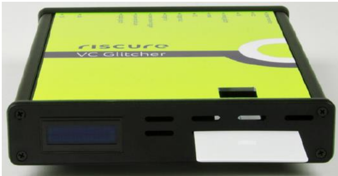
Figure 2. DS1160A Smartcard Voltage and Clock Glitcher with a smart card inserted for testing
