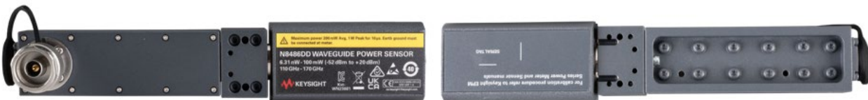
Figure 6. N8486DD-200 comes with built-in EEPROM to store calibration factors with extended dynamic range of -52 to +10 dBm.
